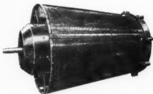
S-A Gilbert Screen with a preliminary scrubbing barrel for a clean, accurately sized product.
